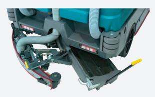
EasyRemove™ debris tray glides in and out on wheels, relieving operators of strain during transport and dumping, and increasing uptime.
