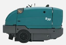
Engineered, fiber-reinforced composite covers are light weight, corrosion resistant, and manufactured with a high-density material. The superior finish makes these covers easy to clean and restorable even if damaged.
