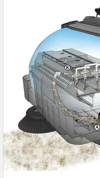
Ensure operator safety, by alerting and shutting down sweeping functions, if increases in hopper temperature are sensed by Thermo-Sentry.™
