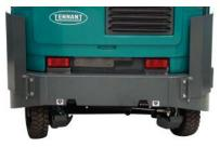
Minimize risk of damage to both the machine frame and the facility with rounded rear corners and rear tower bumpers that improve turn off from structures (walls and racking), while protecting from accidental contact.
