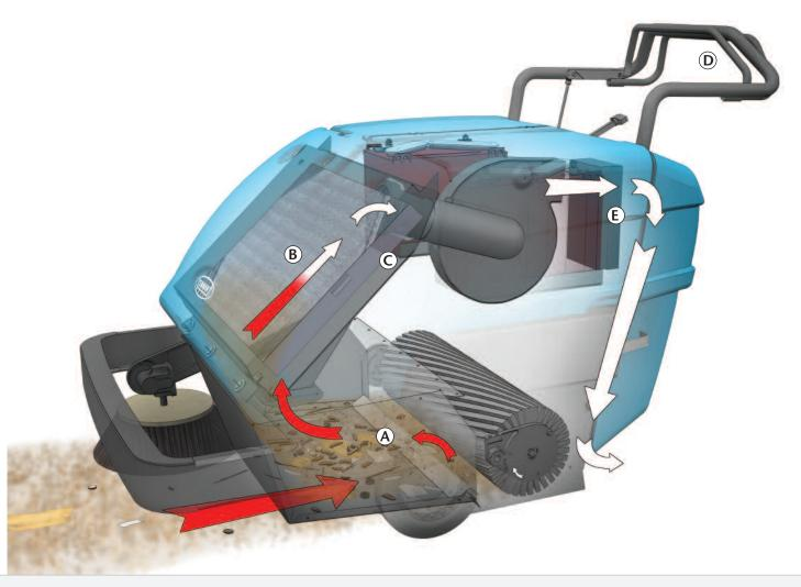
A Large capacity steel hopper – free-floating hopper holds up to 150 lb / 68 kg, 2.8 ft<sup>3</sup> / 79 L of debris.
